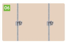
6.Thread the two front wire through the cylindrical screw **f** tting.And tightenthe screws as well.
