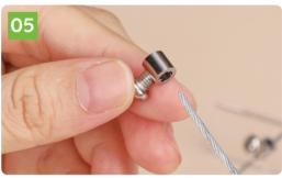
5.Thread the two front wire through the cylindrical screw  ${\bf f}$  tting.And tightenthe screws as well.
